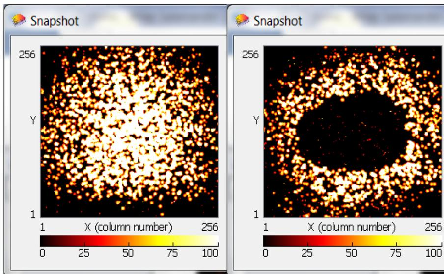
The droplet of water is shown as a black spot containing no alpha particle traces in the picture on the right. A layer of water only 45  $\mu\text{m}$  thick is enough to absorb particles emitted by americium. The drop of water has shielded alpha particles.
